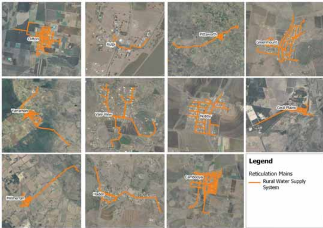
Figure 4.3 Rural Town Water Reticulation Systems
